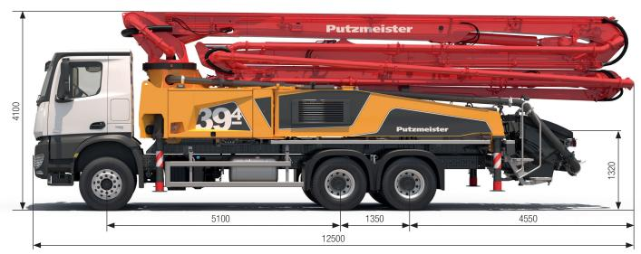
Note: Standard version. Dimensions and weights depend on truck, pump model and equipment. Dimensions in mm for MB-Arocs 3342.
